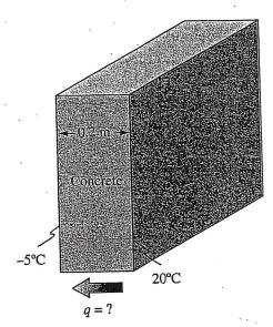
Determine the heat loss through a wall 10 m long and 3 m high
